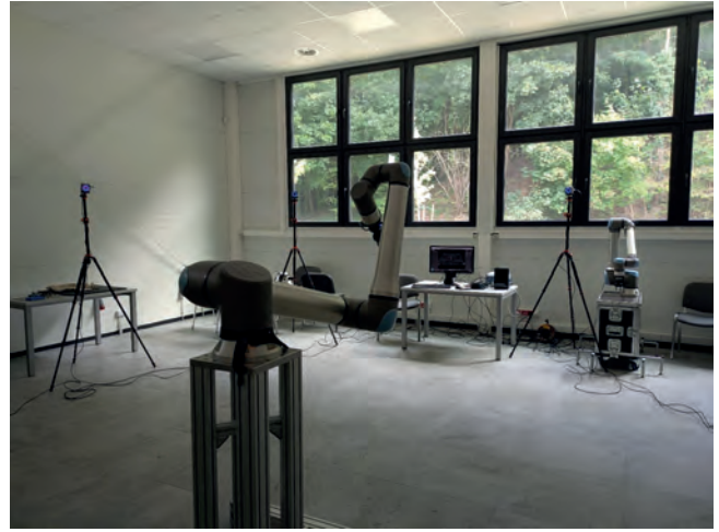
Rys. 2. Robot UR20 i OptiTrack Motion Capture System w laboratorium IIM
