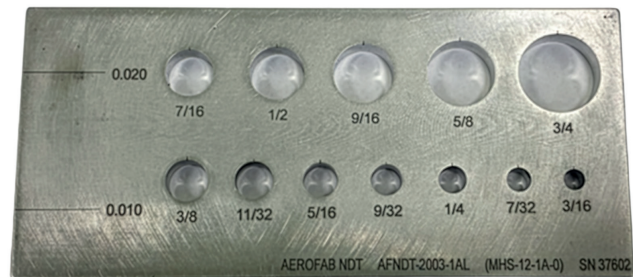
Fot. 3. Wzorec AEROFAB NDT AFNDT-2003-1AL Photo 3. AEROFAB NDT reference standard, model AFNDT-2003-1AL
