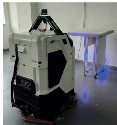
Fig. 11. Experiment setup for navigation test with and without the Hit Layer
