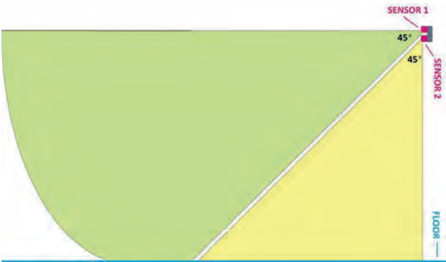
Fig. 2. ToF sensor range (one column of sixteen) Rys. 2. Zakres czujnika ToF (jedna kolumna z szesnastu)
