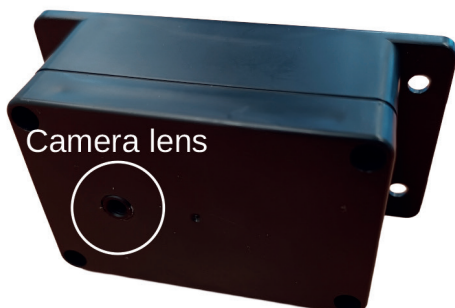
Fig. 16. The assembled and closed in the box device with thermal camera
