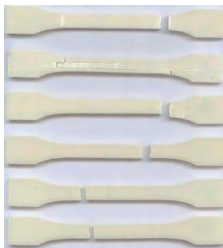
Fig. 2. Collation of samples after tensile strength test. From left: ABS-M30, PC, Ultem 9085. From top: Lengthwise filament distribution (Solid, Sparse, Sparse Double-Dense), Crosswise filament distribution (Solid, Sparse, Sparse Double-Dense)
