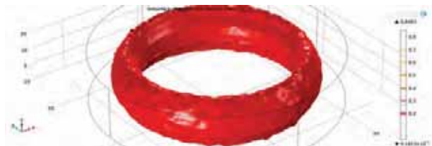
Fig. 1. Magnetic flux density around disc shaped magnet with magnetization M_z
