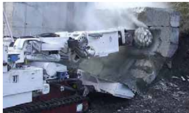
Fig. 7. R-130 roadheader during initial tests at REMAG's testing facility [4]
